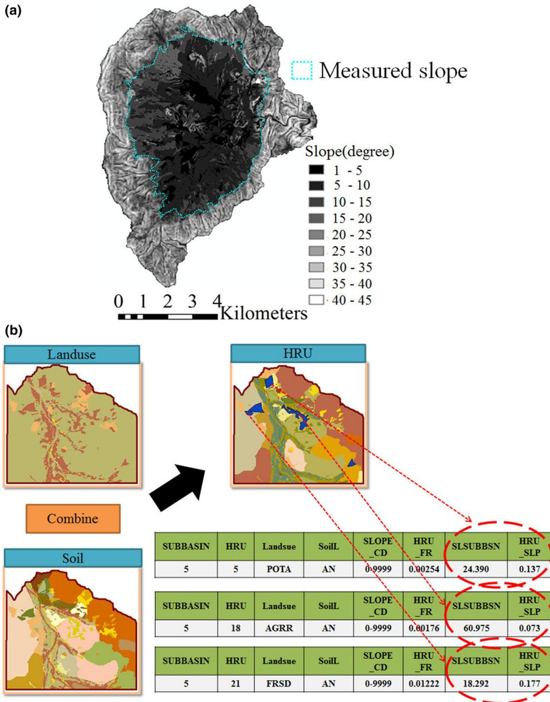
**Fig. 4** The concept of application of the measured slope. **a** Slope in the Hae-an-myeon watershed and **b** measured slope to individual HRU in SWAT
