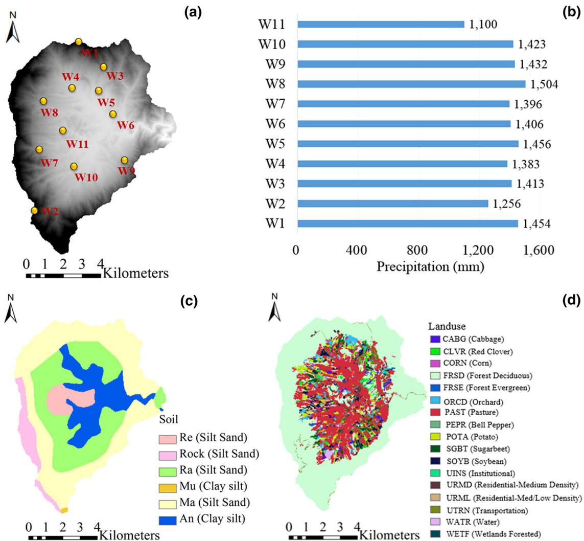
**Fig. 3** SWAT input. **a** Location of weather stations in Haean-myeon watershed, **b** precipitation at 11 weather stations, **c** major soil types in the Haean-myeon watershed, and **d** land use in the Haean-myeon watershed
