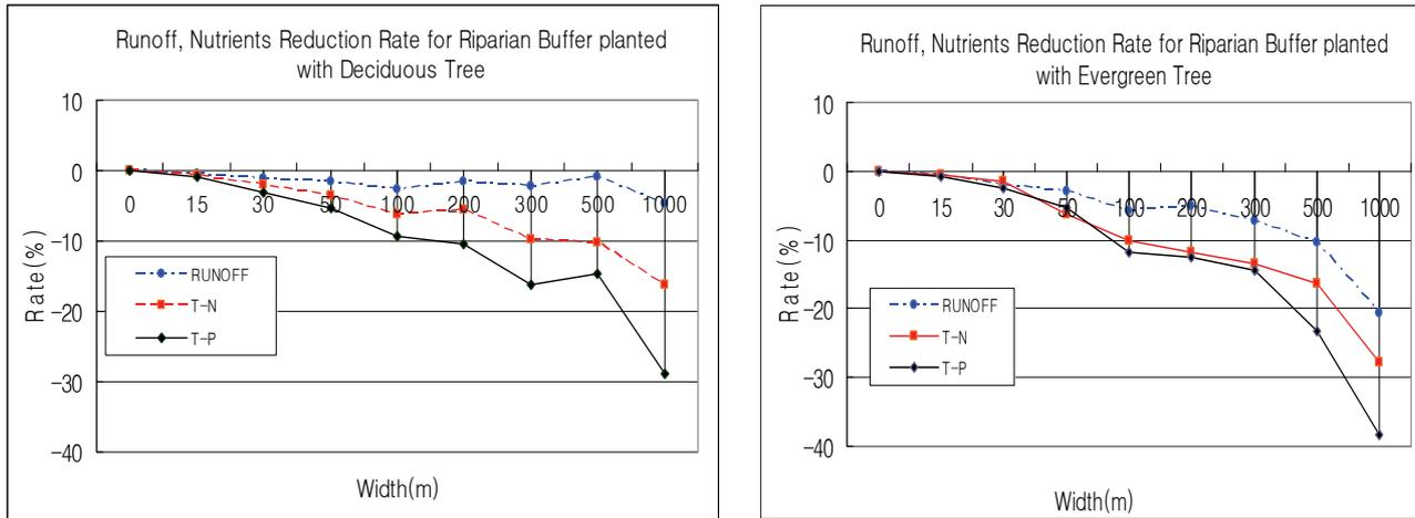
Fig. 10. Changes in flow, T-N, and T-P with riparian buffer width in the Gap Stream watershed
