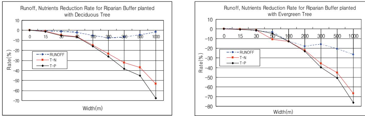
Fig. 8. Changes in flow, T-N, and T-P with riparian buffer width in the Daejeon Stream watershed
