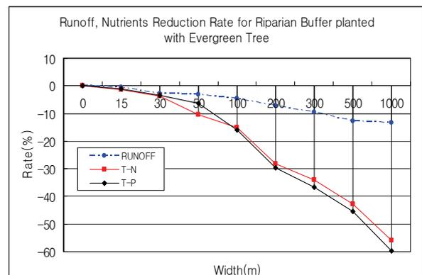
**Fig. 6.** Changes in flow, T-N, and T-P with riparian buffer width in the Yudeung Stream watershed
