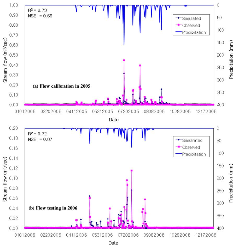
Figure 9. (a) Calibration and (b) testing of daily streamflow for the Bongkok watershed.
