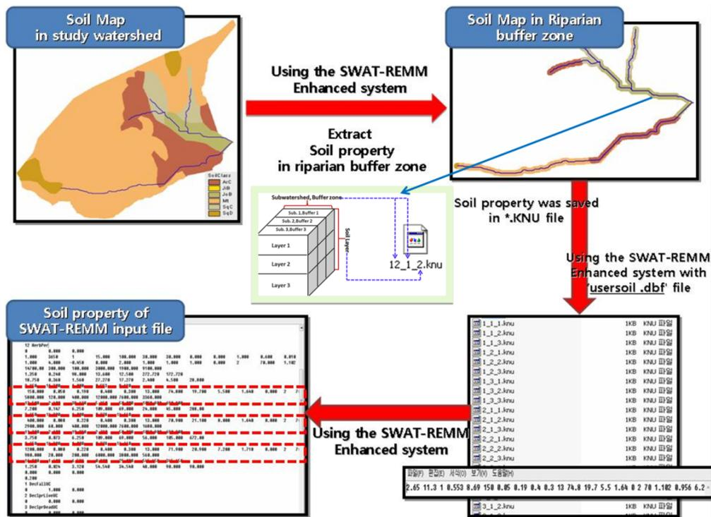
Figure 8. Extraction of soil properties at riparian buffer zone for REMM simulation.
