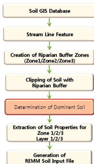
Figure 5. Overview of soil property extraction module in the enhanced SWAT-REM.
