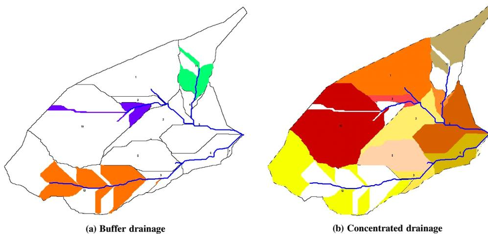
Figure 7. (a) Buffer drainage and (b) concentrated drainage delineated using enhanced SWAT-REM.
