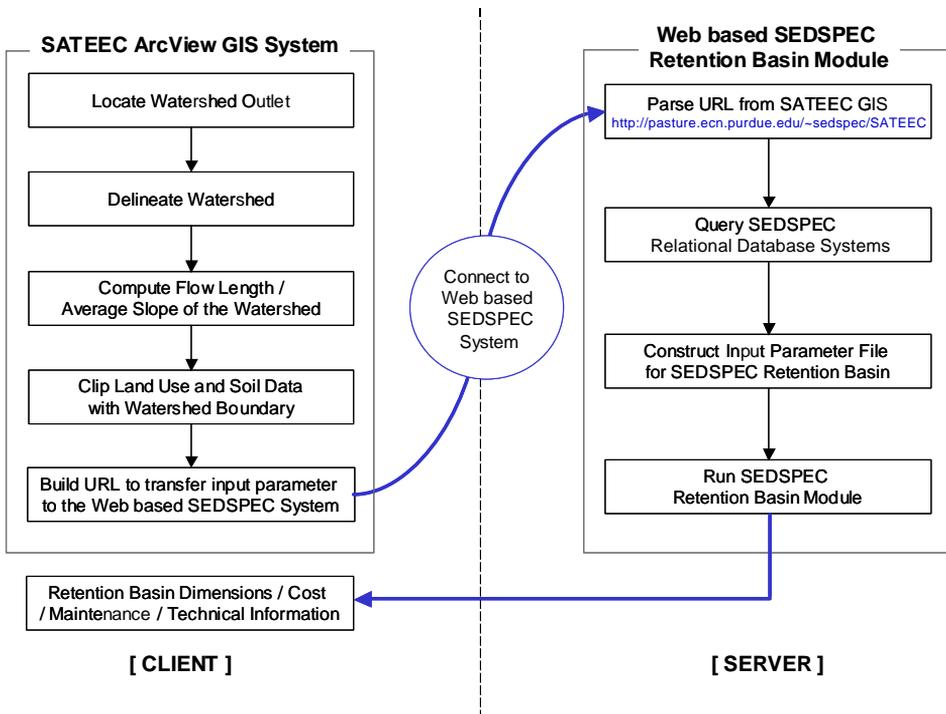
Fig. 3. Interface to the Web-based SEDSPEC from the SATEEC GIS system.
