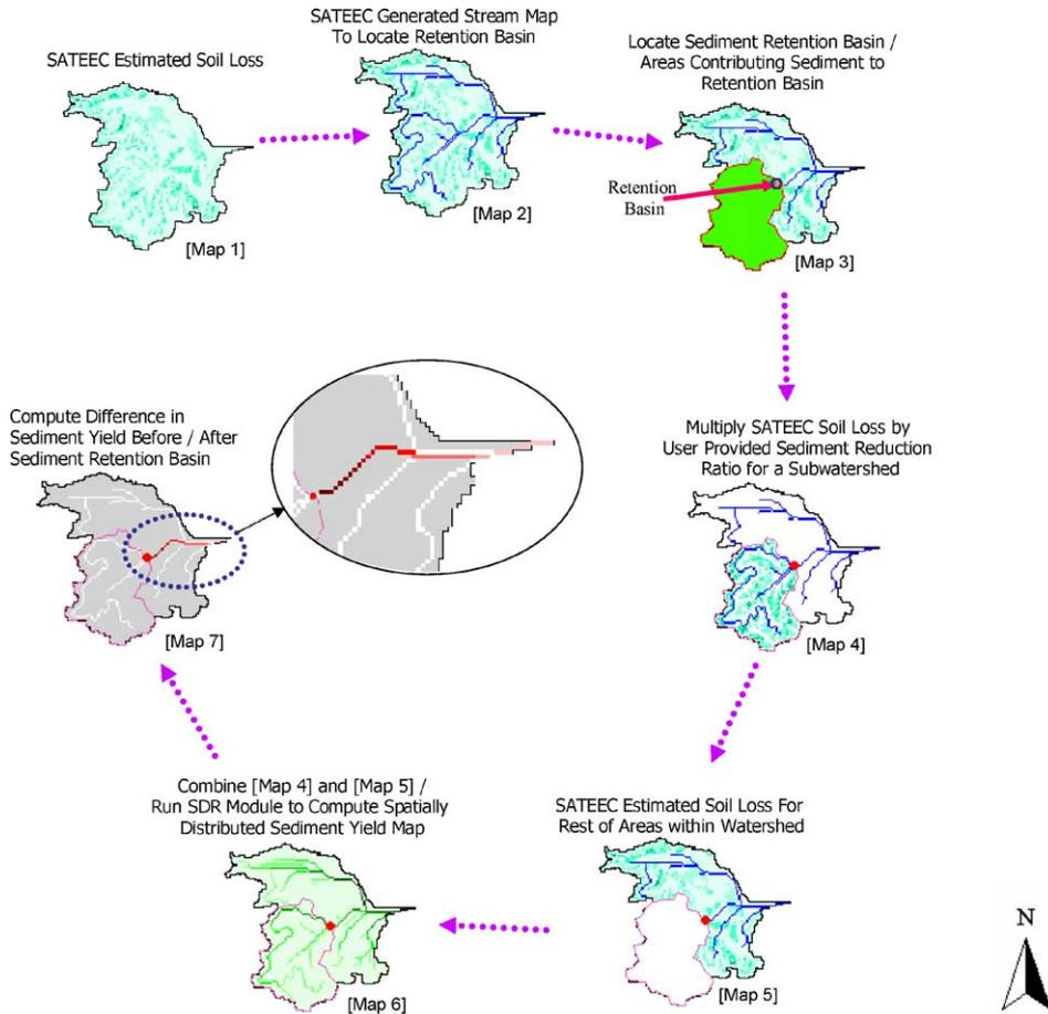
Fig. 2. How SATEEC estimates the effects of sediment retention basins on downstream water bodies.
