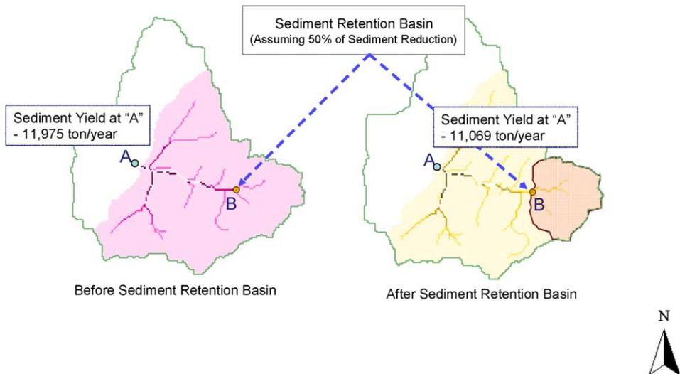
Fig. 7. Effect on downstream water bodies of the sediment retention basin.
