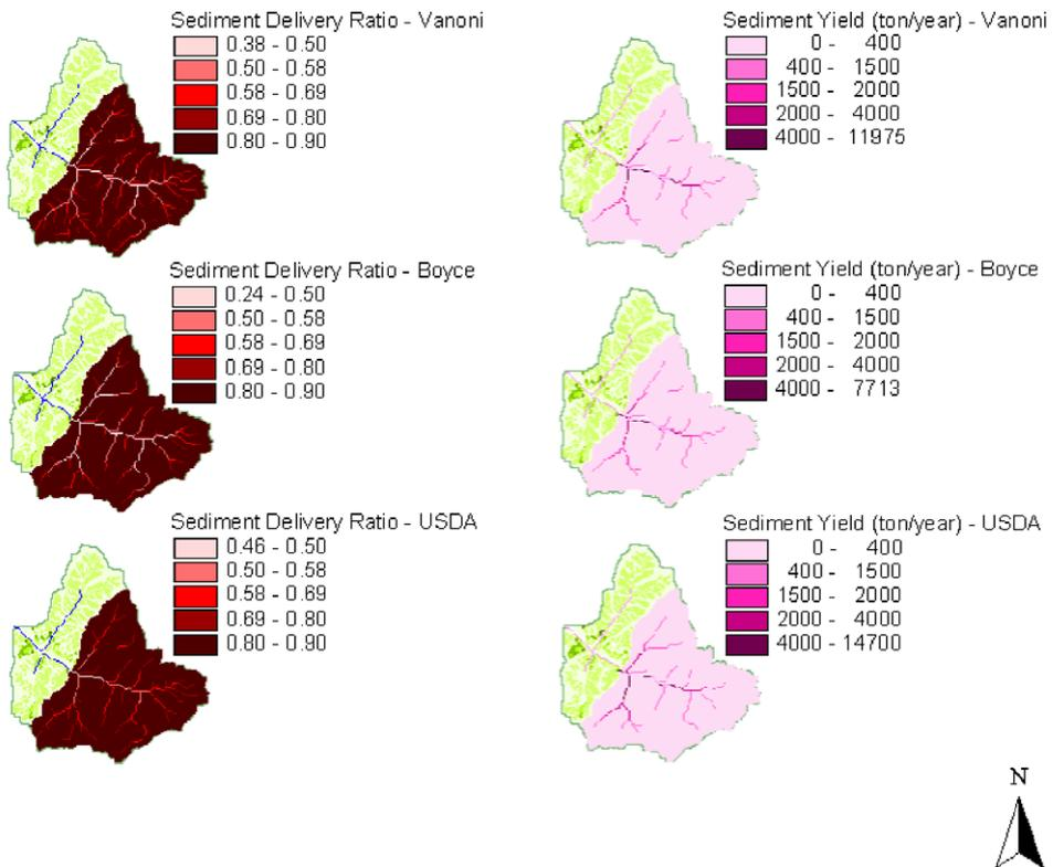
Fig. 6. SATEEC estimated spatially distributed sediment delivery ratio and sediment yield maps (cell values represent the SDR and sediment yield for watershed having that cell as an outlet).
