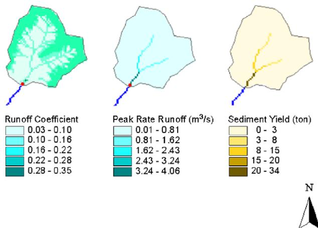
Fig. 8. Spatially distributed sediment yield from a single storm event (cell values in each map represent the runoff coefficient, peak rate of runoff and sediment yield for a watershed having that cell as an outlet).
