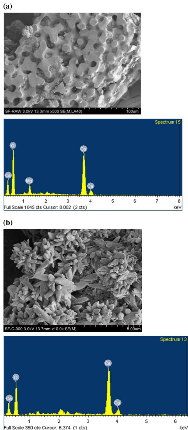
**Fig. 2** SEM-EDX results of the NSF (a) and CSF\_900 (b) samples
